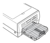
4 Push both the right and left eject buttons to open the main cover.
